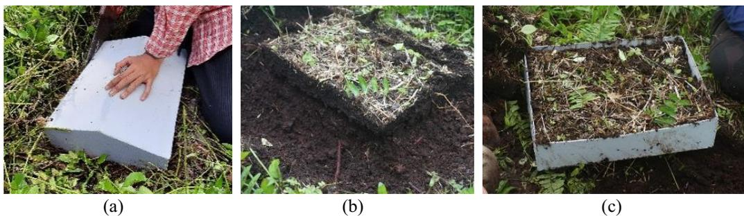
**Figure 2.** Step-by-step soil collection for lysimeter: (a) measure a 40 x 30 cm area, (b) cut the soil with a saw and dig around it, and (c) collect the soil in the same volume as the lysimeter and place it in the container.
