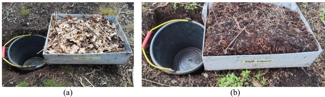
**Figure 3.** (a) Lysimeter setup including decomposed cover crops placed above the peat soil, and (b) lysimeter containing only peat soil. Below each lysimeter setup, a bucket is positioned to collect leachate following each rainfall event.
